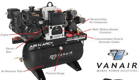
This Air N Arc® 150 provides you with three forms of power in one compact and economic unit, allowing you to save space and weight on your vehicle. Provides up to 190 amps of welding power and a 30 gallon air reservoir tank.
